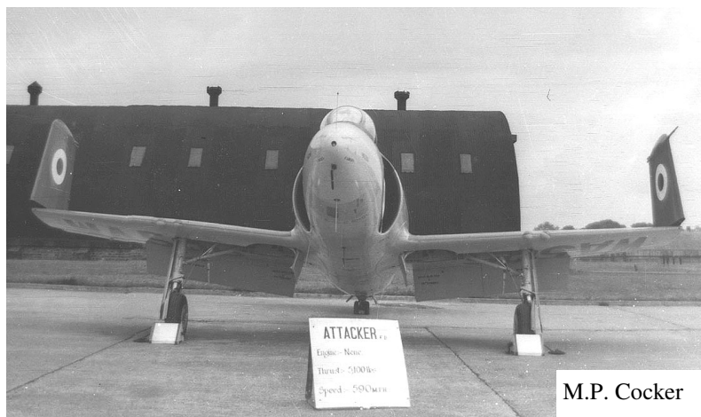
ATTACKER. Vickers Supermarine. 1953/1957 590 m.p.h. The first frontline jet of the Royal Navy it was developed from the prototype Spiteful which was supposed to have been a replacement for the Spitfire.
