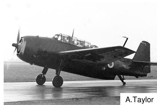
AVENGER. Grumman, U.S.A. 1953/1954. 270 m.p.h. A three-seat torpedo bomber with the power and strength needed by the Fleet Air Arm in 1943 to operate from carriers.
